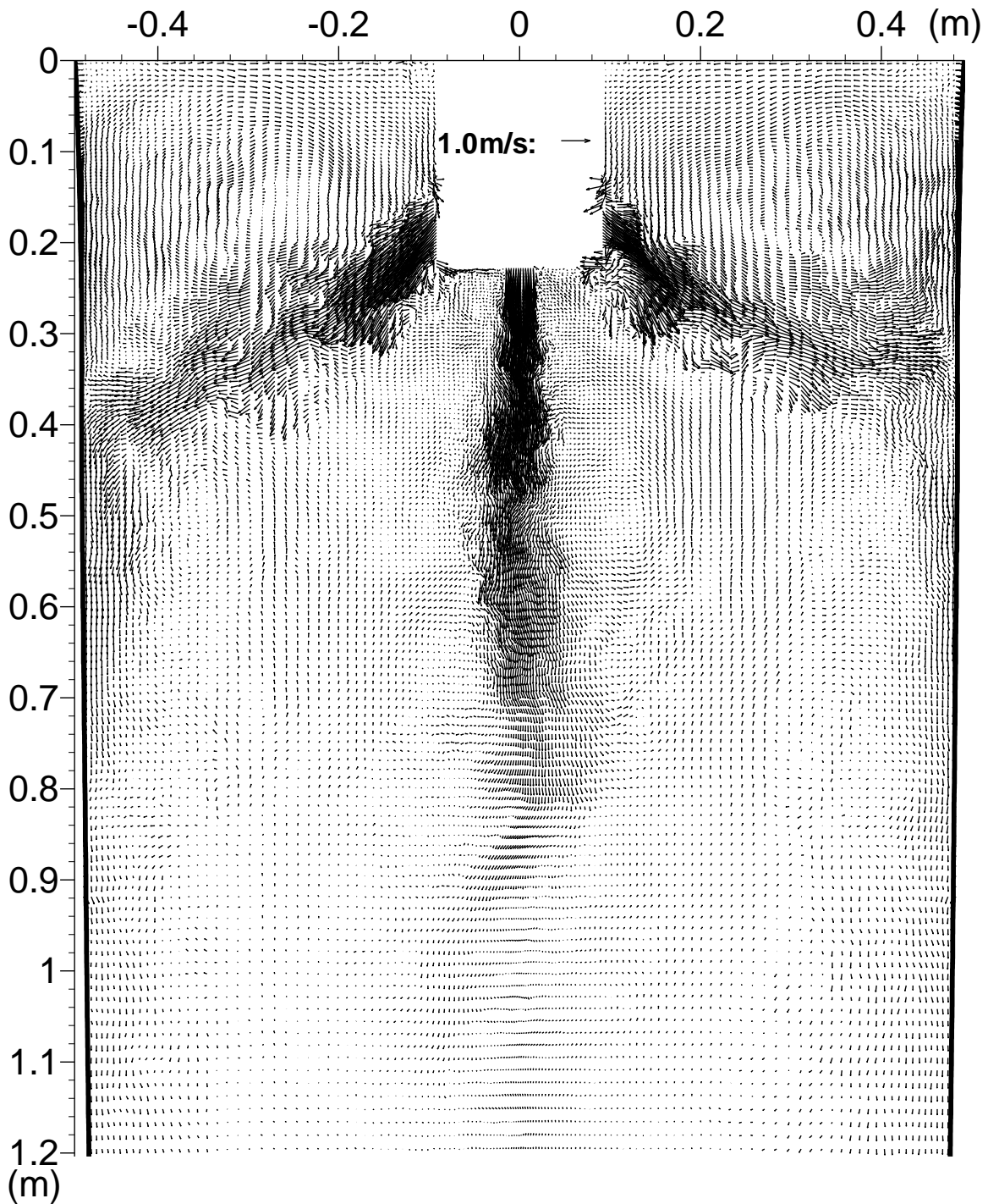
Fig. 4. Typical instantaneous velocity vector plot computed at the center plane between wide faces [11] (Animation 4).
